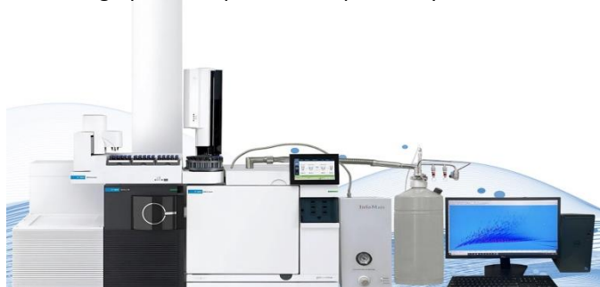
Figure 3. Model L10 installed on an Agilent GC/QTOF system, demonstrating practical integration with a commercial GC-MS platform.
