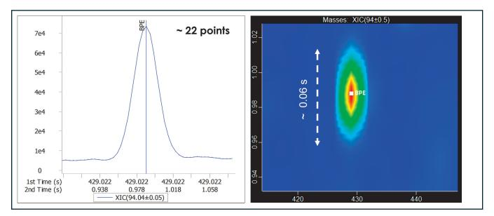
Figure 2. Extracted ion chromatogram (XIC) at m/z = 94.04  $\pm$ 0.05 of BPE at target dosage level of 1%, corresponding to 0.095 mg/L. BPE has peak width at base (wb) of ~0.06 s.
