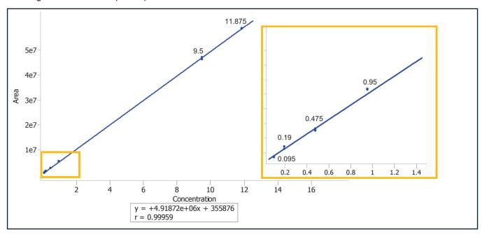
Figure 3. Linearity of BPE for 1-125% dosage level corresponding to 0.095 to 11.875 mg/L of BPE.
