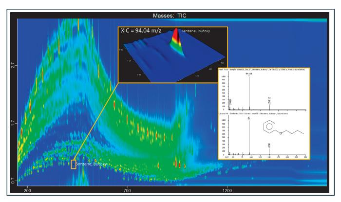
Figure 1. Total ion chromatogram (TIC) for BPE detection and mass spectral confirmation in a spiked commercial diesel B7.
