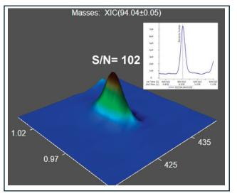
Figure 4. BPE signal-to-noise (S/N) recorded at 0.095 mg/L.
