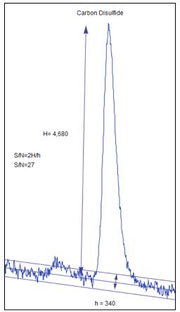
**Figure 3.** Signal-to-noise determination for the analysis of 1.24 ppm CS<sub>2</sub> in 1-propanol using the Polyarc System.
