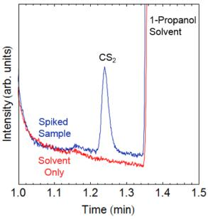
**Figure 2.** Polyarc/FID chromatogram for the analysis of  $1.24 \text{ mg/kg } \text{CS}_2$  in 1-propanol (blue) and a solvent-only blank (red).
