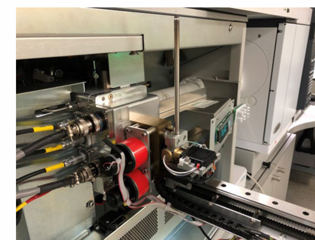
DIP loading position
