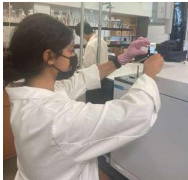
Figure 3. Image of fiber injection in GC inlet.
