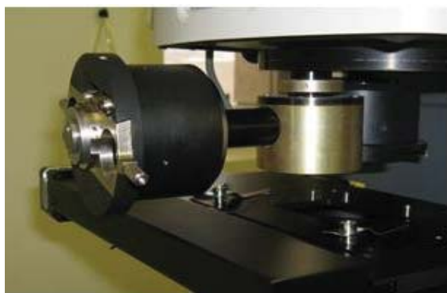
Figure 1. Top: Schematic of the patented Agilent Large Sample Microscope Objective accessory. Bottom: Photograph of the Large Sample Microscope Objective accessory.
