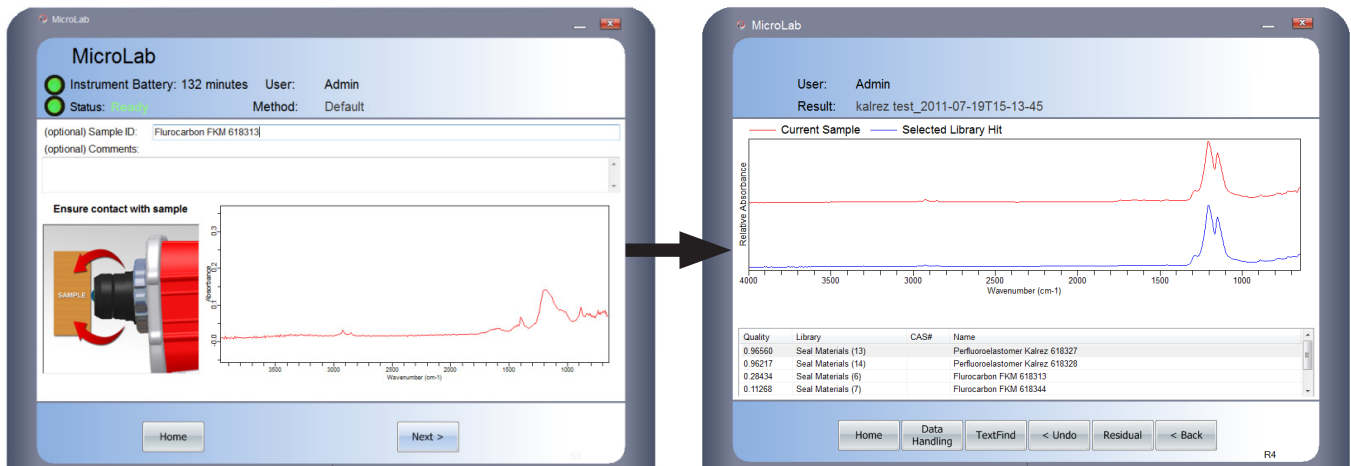
Figure 3. Sample is lightly pressed against spherical Ge ATR element (left) and real time display instantly shows that adequate contact is made. Co-addition is initiated and resultant high quality spectrum is searched against onboard spectral library (right).
