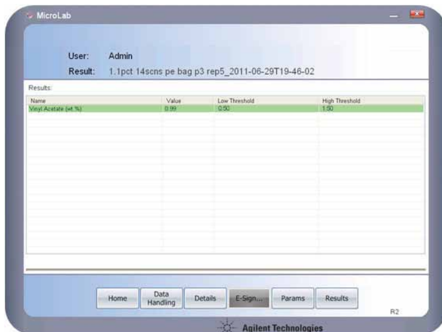
Figure 7. The result for the 1% VA validation standard — green color indicates an in-spec sample
