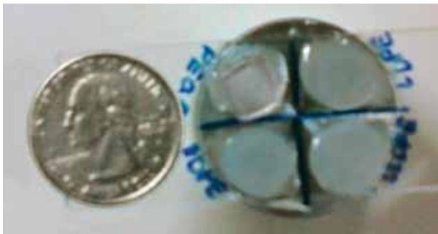
Figure 1. Four polyethylene samples, mounted for testing.
