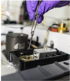
Figure 1. Installation of the Jetanizer™ into an FID.
