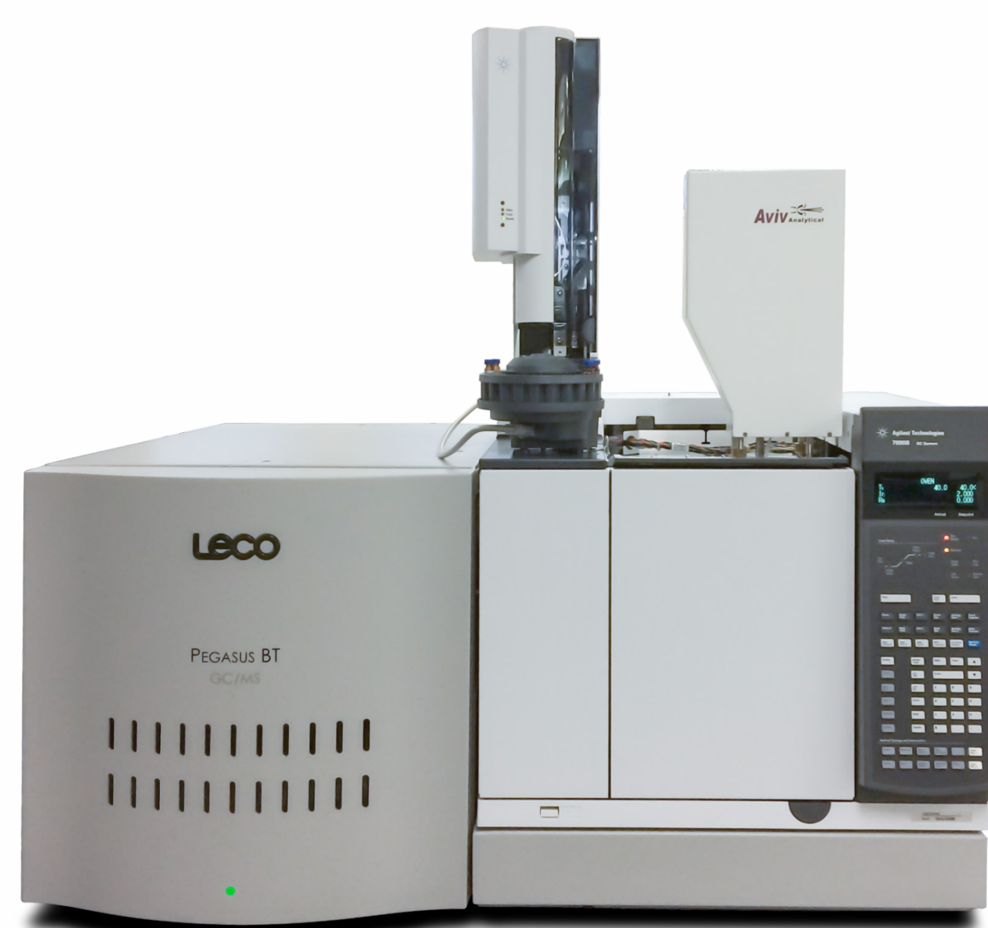
Figure 1. Instrument Configuration: Agilent 7890GC with the Aviv Analytical Fast GC mounted onto the detector port, and the Pegasus BT GC-TOFMS pre-production prototype with increased maximum scan speed from 50 to 100 spectra/second.
