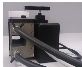
Fig. 1 Batch Cell (with temperature control function)
