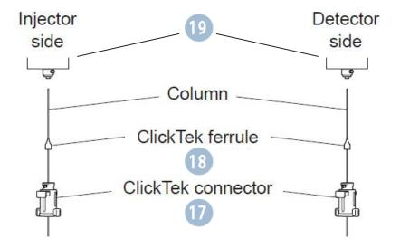
Capillary Column Insertion Depth (measure from tip of ferrule to end of column)<sup>1-3</sup>
