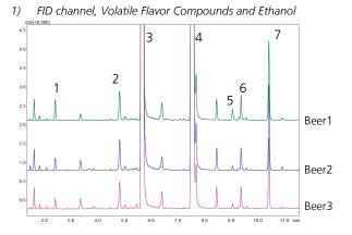
Figure 5: Chromatograms of VOCs in three different beer samples. Compound of interest: 1. Acetaldehyde 2. Ethyl acetate 3. Ethanol 4. *n*-Propanol (ISTD for Ethanol) 5. *iso*-Amyl acetate 6. *n*-Butanol (ISTD for VOCs) 7. *iso*-Amyl alcohol.
