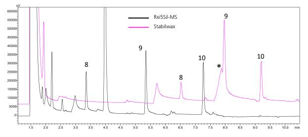
Figure 7: Chromatogram of VDK standard in ECD channel on either Rxi-5Sil MS or Stabilwax column. Compounds of interest: 8. Diacetyl (2,3-butanedione) 9. 2,3-pentanedione 10. 2,3-hexanedione (ISTD for VDKs). \* denotes a non-analyte peak present in blank.
