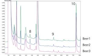
Figure 6: Chromatograms of VDKs in three different beer samples. Compound of interest: 8. Diacetyl (2,3-butanedione) 9. 2,3-pentanedione 10. 2,3-hexanedione (ISTD for VDKs).
