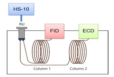
Figure 1: Schematic drawing of the dual column configuration for the Shimadzu Beer 3-in-1 Analyzer.
