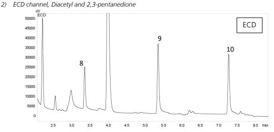
Figure 3: Chromatogram of VDK/VOC calibration standard in ECD channel. Compounds of interest: 8. Diacetyl (2,3-butanedione) 9. 2,3-pentanedione 10. 2,3-hexanedione (ISTD for VDKs).
