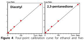
Figure 4: Four-point calibration curve for ethanol and fivepoint calibration curves for VOCs and VDKs. Concentrations of analytes and internal standards were as described in methods.
