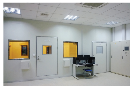
Figure 1. Typical human calorimeter chamber (courtesy of Fuji Medical Science).
