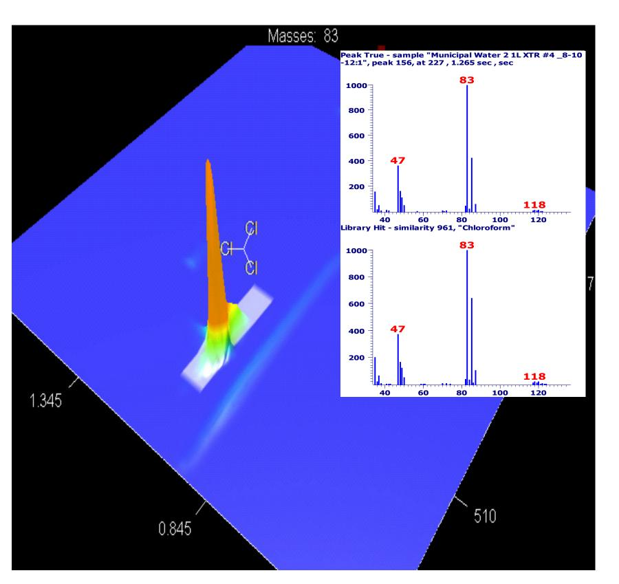
Figure 4. A six-point calibration curve was developed for chloroform from 46.4 pg to 24.7 ng. The concentration of the chloroform peak found in a 1 liter municipal water sample shown in the contour plot is back calculated to be 1.57  $\mu$ g/L or 1.57 ppb.
