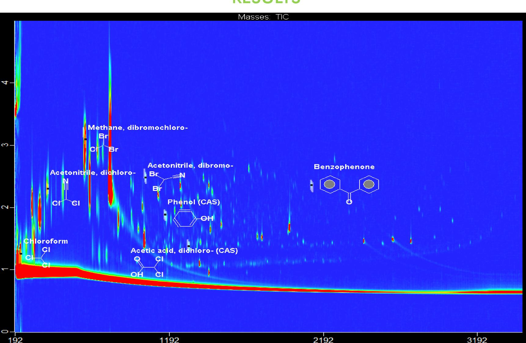
Figure 1. Two-dimensional contour plot chromatogram of a 1 liter municipal water sample prepared by solid-phase extraction
