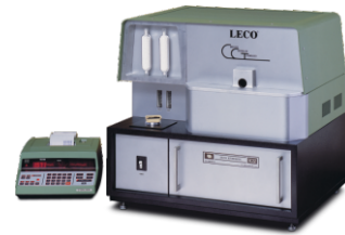
1979: The SC-32, the industry's first automated sulfur analyzer, replaces the tedious ESCHA wet chemistry method.
