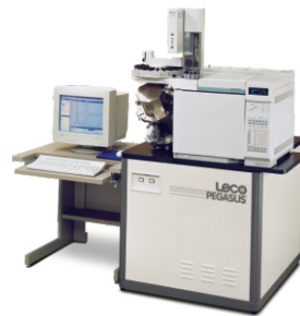
1997: The Pegasus ® GC-TOFMS, one of the first time-of-flight mass spectrometers in the marketplace, is released by LECO.
