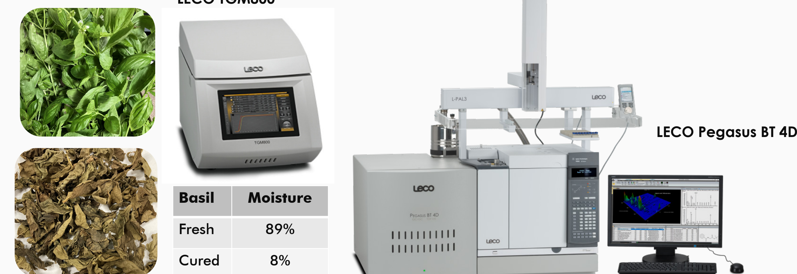
Figure 1. Fresh and cured basil were analyzed. The moisture level in the samples was measured with LECO's TGM800 and aroma profiling was done with LECO's Pegasus BT 4D.
