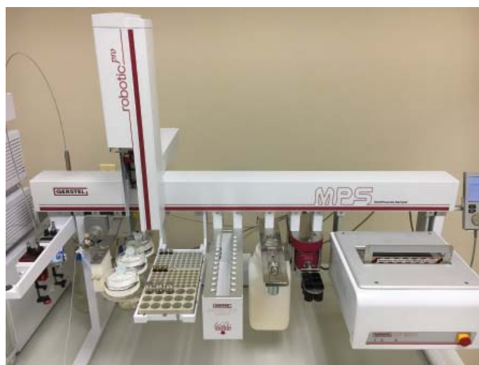
Figure 1. MPS robotic PRO Multi-Purpose Sampler with the GERSTEL QuickMix, CF-200 centrifuge, and Universal Filtration option.
