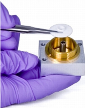
Orientation of the collector and insulators in the FID
