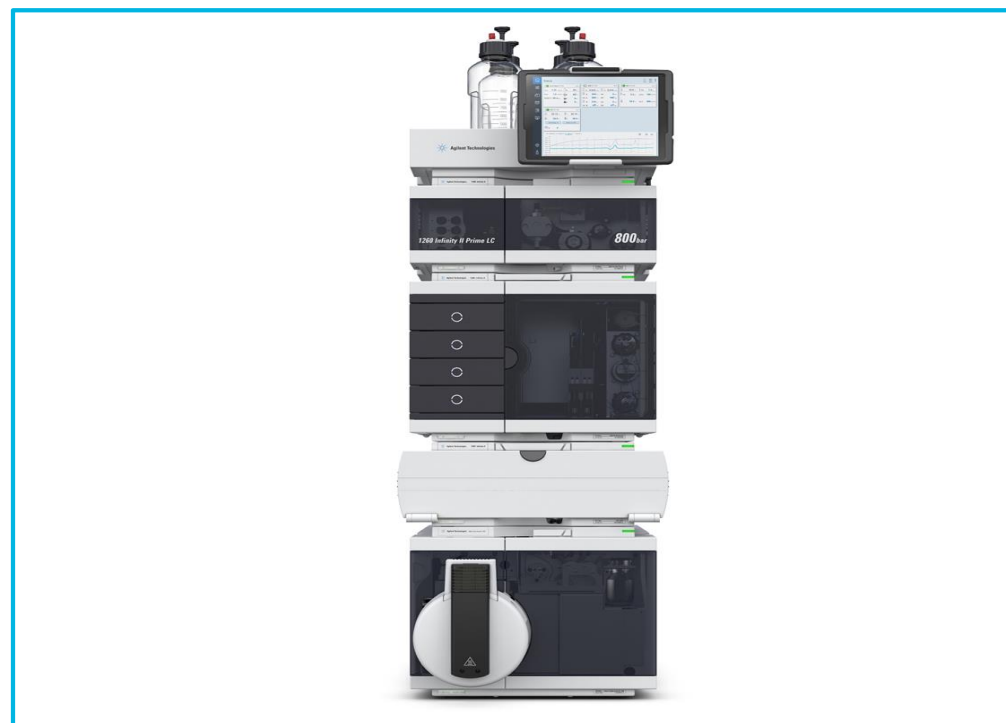
Figure 2. The smallest LC/TQ in the world—Agilent Ultivo LC/TQ
