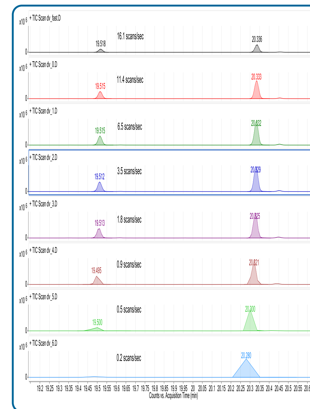
Figure 5: Chromatogram of the same essential oil at different scan acquisition rates
