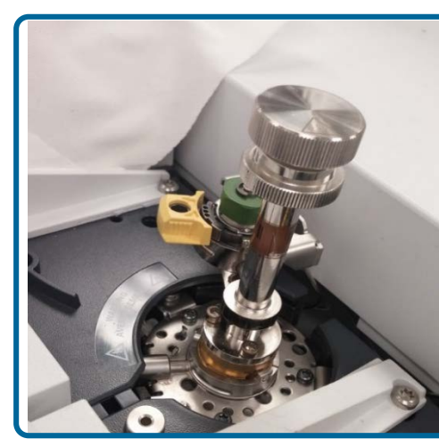
Figure 2: The TSP inserted into the GC Inlet
