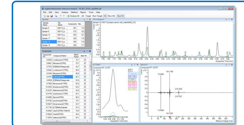
Figure 5. Accurate mass metabolomics screening in Unknowns Analysis. On average, more than 100 hits from the accurate mass metabolomics PCDL were detected in each sample. The novel profile-based algorithm is also capable of extracting features with high quality spectra and accurate mass from highly saturated regions of the chromatogram, where conventional deconvolution algorithms typically fail (figure 6).
