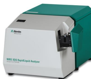
Fig. 1: The NIRS XDS RapidLiquid Analyzer was used for spectral data acquisition over the full range from 400 to 2500 nm.
