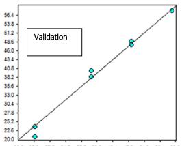
20.0 23.9 27.8 31.7 35.6 39.5 43.4 47.3 51.2 55.1 59.0 Figure 4: Values calculated from the validation NIR spectra vs. lab values for the percentage of embedded water measurement in soft contact lenses.
