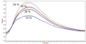
Figure 2: NIR spectra (with SNV) of the water absorption in soft contact lenses with 24%, 38%, 48%, and 58% embedded water.
