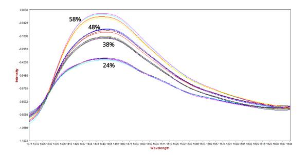
This application note describes the determination of water content in soft contact lenses by NIRS. Using a liquid sample kit with a gold diffuse reflector, the soft contact lenses were analyzed in transflection mode. A PLS model for regression was built to predict the water content.
