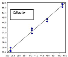
Figure 3: Values calculated from NIRS data using a PLS model vs. lab values for the percentage of embedded water measurement in soft contact lenses.
