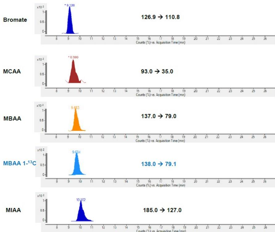
Highly sensitive and selective trace analysis of disinfection byproducts: Extracted Ion Chromatograms of 50 µg/L MBAA (monobromoacetic acid) 1-<sup>13</sup>C (internal standard), bromate, MCAA (monochloroacetic acid), MBAA (monobromoacetic acid), and MIAA (monoiodoacetic acid), respectively (further chromatograms and results see below)
