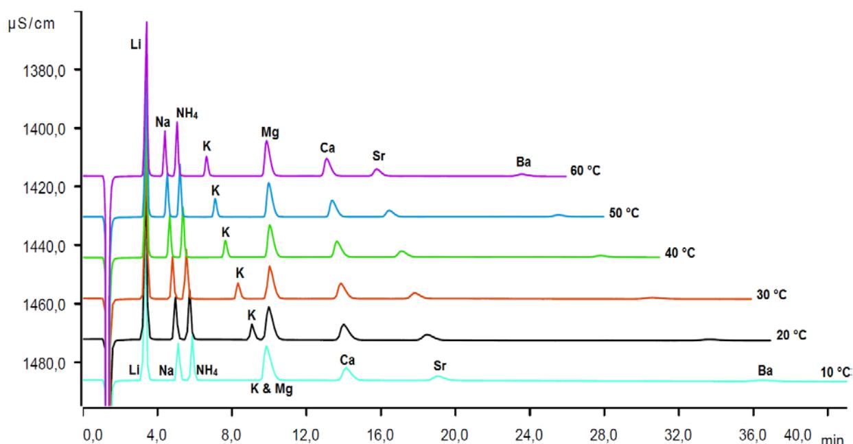
Column temperature influences the separation time of cations on the Metrosep C 6 - 150/4.0 high-capacity column. Increasing temperature only slightly reduces the retention time of lithium, sodium, ammonium, magnesium, and calcium. By contrast, increasing temperature significantly reduces retention times for potassium, strontium, and barium. This dependence allows to optimize ammonium, potassium, and magnesium separation by reducing analysis time for strontium and barium.
