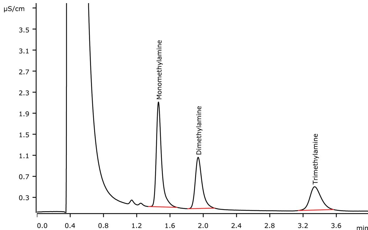
Fast IC means short runtimes and high sample throughput on columns with relatively high flow rates and the standard eluent. The separation and determination of mono-, di-, and trimethylamine is accomplished within four minutes using Metrosep C 4 - 150/2.0.
