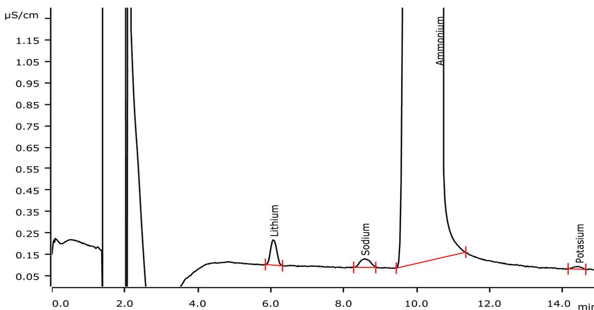
Metrohm Inline Preconcentration Technique with Matrix Elimination (MiPCT-ME) is a powerful tool that combines preconcentration, matrix elimination, and multilevel calibration. In this application, the methodology is applied to the determination of trace sodium besides 2 mg/L of ammonium. The Metrosep C 6 - 250/4.0 column is used for selectivity reasons.
