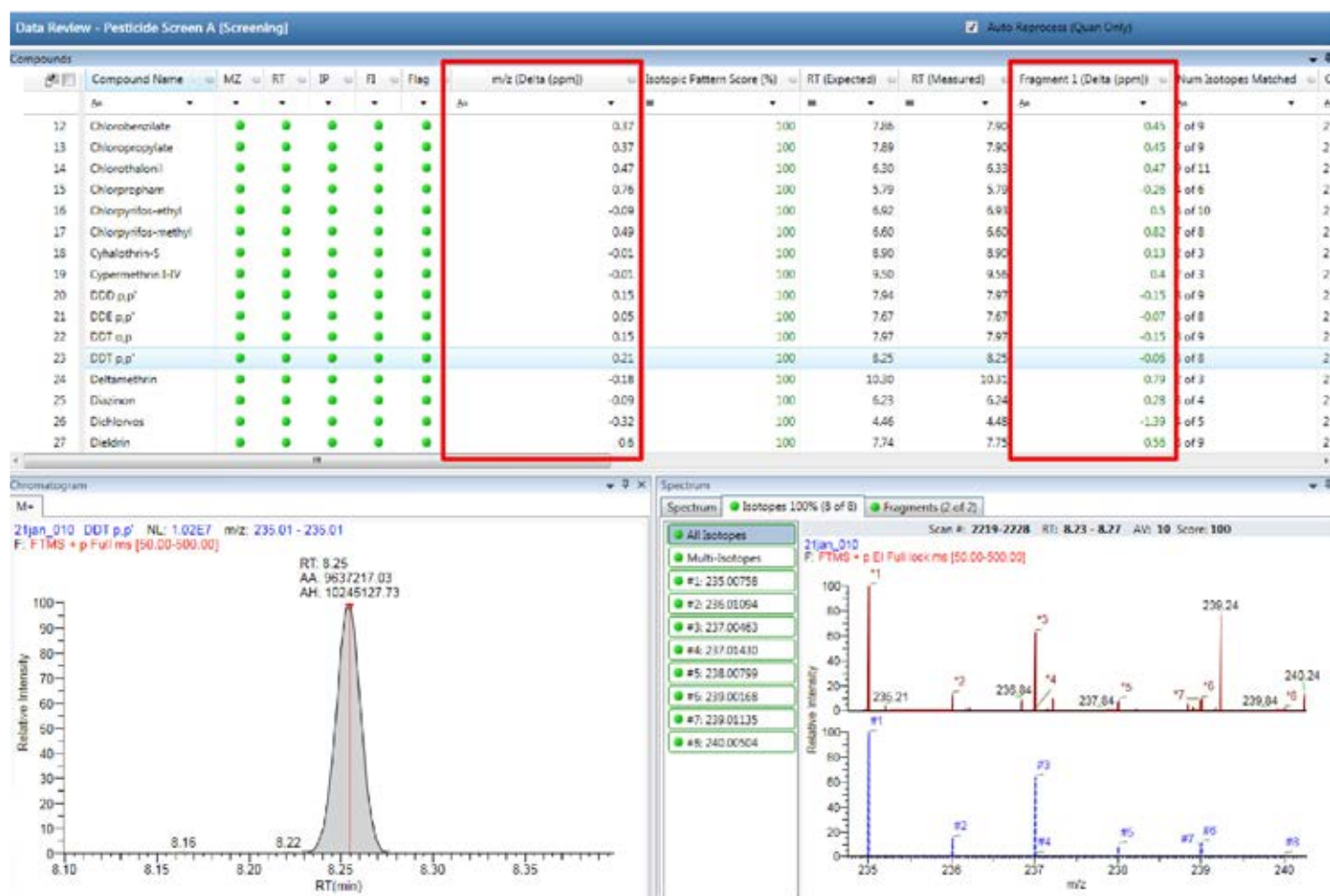
Figure 3. TraceFinder screening browser showing positively identified pesticides (p,p'-DDT as an example) in wheat spiked at 10 ng/mL, based on accurate mass confirmation ( \pm 2 ppm mass window), retention time (RT), isotopic pattern (IP), fragment ions (FI). Sub-ppm mass accuracy for both main and confirmatory ions is highlighted in red boxes.
