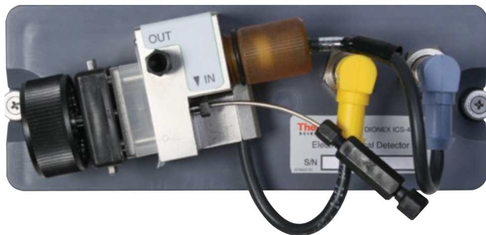
Electrochemical detector cell for applications on standard bore and microbore size columns.
