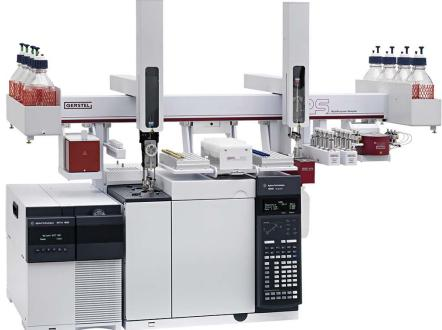
**Figure 1.** Setup used for the automated analysis of blood serum for THC and metabolites. Dual Head MultiPurpose Sampler (MPS) equipped with solvent bottle holder, agitator, standard wash station, trays for eluate vials, SPE cartridges and samples, SPE module, two solvent filling stations (SFS), MultiPosition eVAPoration station (mVAP) and solvent bottle holder (from left to right).
