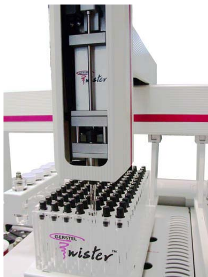
Figure 1. Sample rack of MPS2-TDU with a capacity of 98 positions; Twisters are put in a clean empty glass liner and capped with a special tube head.
