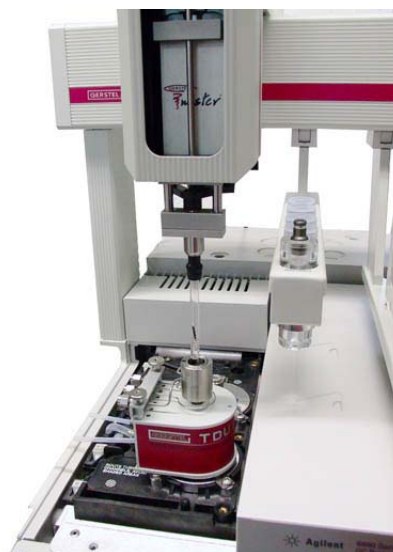
Figure 2. MPS-2-TDU-CGC-MS setup; The MPS-2 robot inserts the liners into the TDU for thermal desorption.
