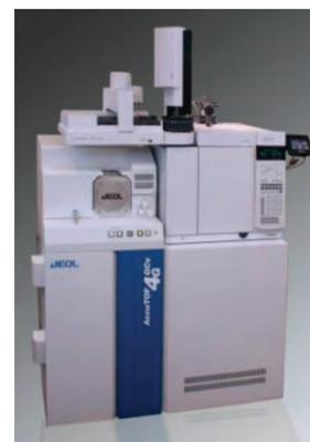
Figure 1. JMS-T100GCV AccuTOF GCv 4G GCxGC/HR-TOFMS system
