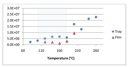
Figure 2 – Temperature Profile Plot of the Acetaldehyde Peak Area for the Tray Sample (blue diamond) and the Film Sample (red triangle). The grey box indicates the cooking temperature range from 100°C (212°F, boiling water) to the manufacturer's upper oven limit of 177°C (350°F)
