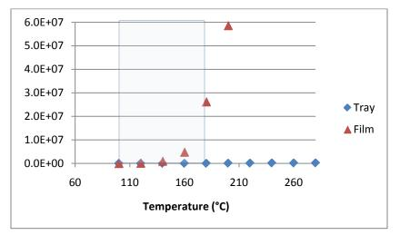
Figure 4: Temperature Profile Plot of the Chloromethane Peak Area for the Tray Sample (blue diamond) and the Film Sample (red triangle). The grey box indicates the cooking temperature range from 100°C (212°F, boiling water) to the manufacturer's upper oven limit of 177°C (350°F)
