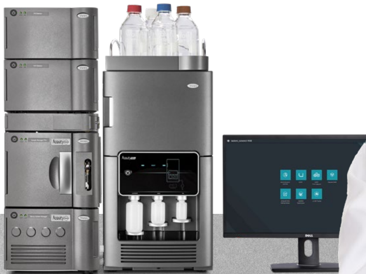
The BioAccord System with ACQUITY™ Premier. The ACQUITY Premier technology contains flow paths, frits, and columns with MaxPeak™ High Performance Surfaces (HPS) to reduced metal surface adsorption of analytes.
