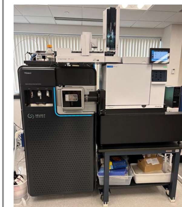
Figure 1. The SELECT SERIES Cyclic IMS fitted with the APGC source.
