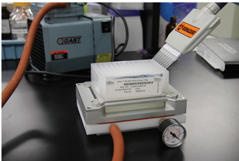
Figure 1. Typical setup for Ostro Pass-through Plate for analysis of milk.
