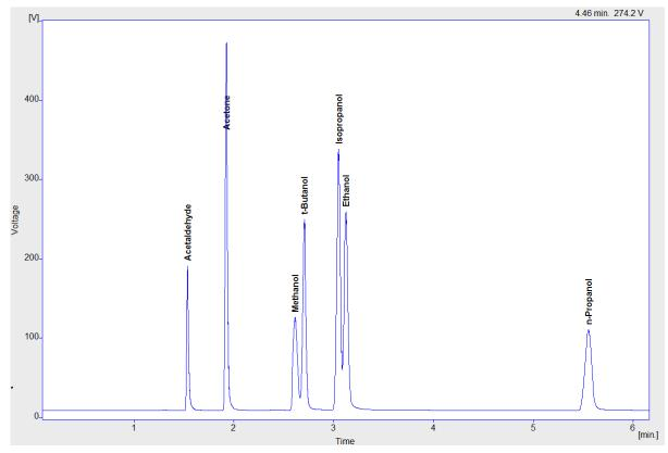
Figure 1: Chromatogram of a 0.05% (w/v) Standard Solution of Acetaldehyde, Acetone, Methanol, t-Butanol (IS), Isopropanol, Ethanol, and n-Propanol (IS)
