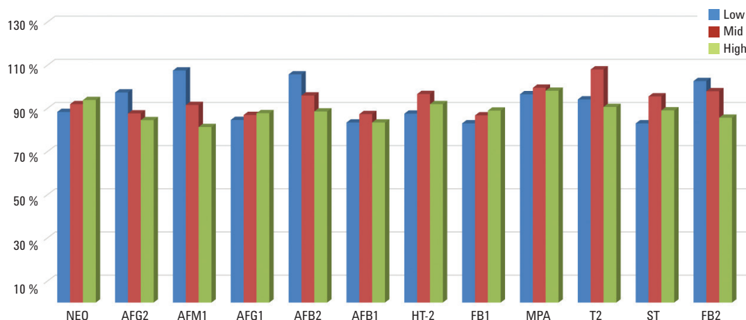
Figure 4. Recovery for 12 mycotoxins in peanut using Agilent EMR—Lipid cleanup. Low: 4 ng/g for aflatoxins (B1,B2,G1,G2,M1), 20 ng/g for other mycotoxins. Mid: 8 ng/g for aflatoxins (B1,B2,G1,G2,M1), 40 ng/g for other mycotoxins. High: 20 ng/g for aflatoxins (B1,B2,G1,G2,M1), 100 ng/g for other mycotoxins.
