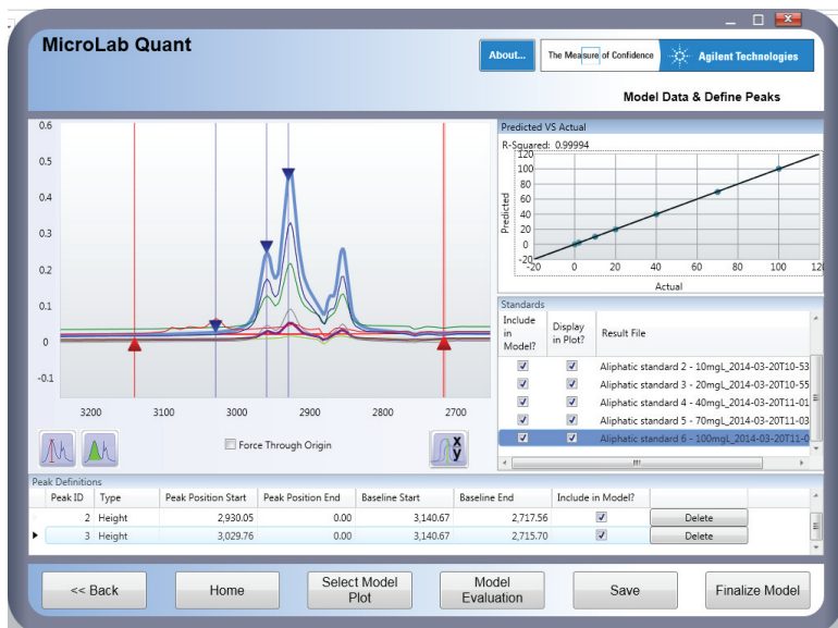
Figure 3. Agilent MicroLab Quant band definition screen allows easy definition of peaks by dragging the peak icon to the appropriate location. The calibration plot in the upper right corner automatically updates, making it easy to optimize peak locations.
