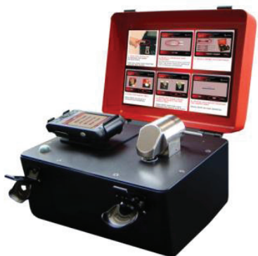
Figure 1. Agilent 4500 Series FTIR, a battery powered, portable FTIR, equipped with 100- \mu\text{m} pathlength TumbIIR sample interface for the measurement of ^2\text{H}_2\text{O} .
