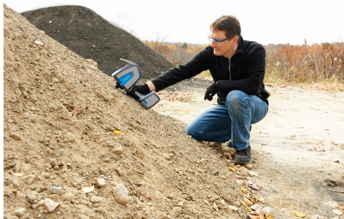
Figure 1b. Agilent 4300 FTIR system being used in the field.
