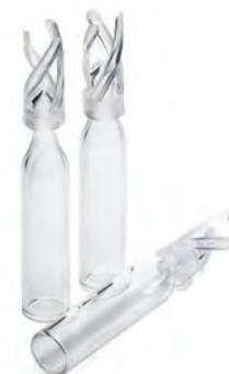
250 µL conical insert with polymer feet, 8010-0131
