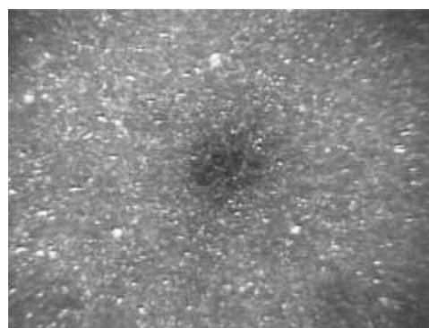
Figure 5. CCD image of the BaTiO 3 disk after laser irradiation showing minimal damage (laser diameter was 10 μm).
