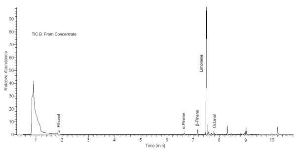
Figure 2: TIC of orange juice from concentrate
