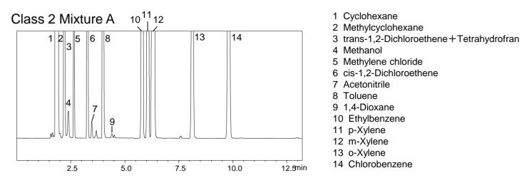
Fig. 2: Water-Soluble Articles, Procedure B, Class 2 Mixture A Standard Solution Chromatogram
