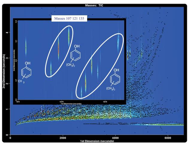
Substituted Phenols may be chromatographically resolved from other compounds in Diesel by the use GCxGC-TOFMS.
