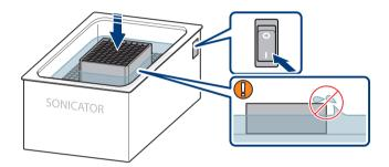
3. Carefully lower the Manifold into the container and sonicate for 5-10 minutes.
