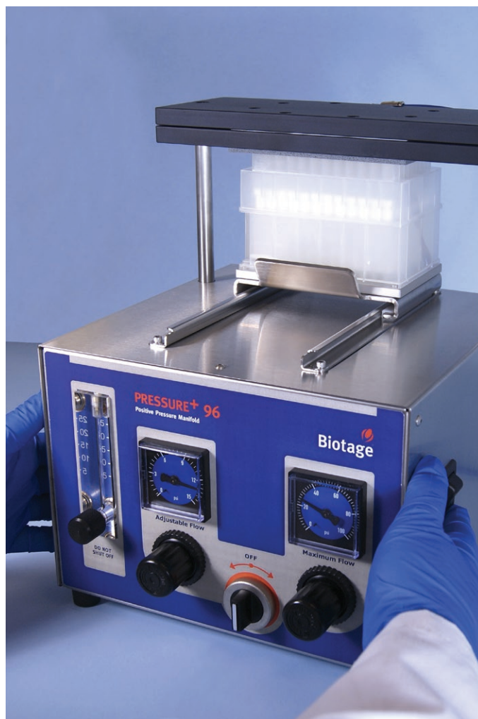
Figure 2. Lower the manifold by pressing down on the two rocker switches simultaneously for approximately 3 seconds.
