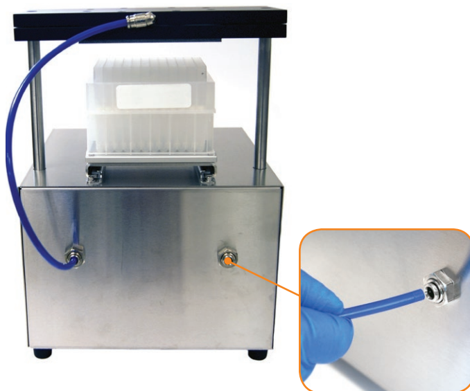
Figure 1. Connect the gas line to the right port at the back of the unit.
