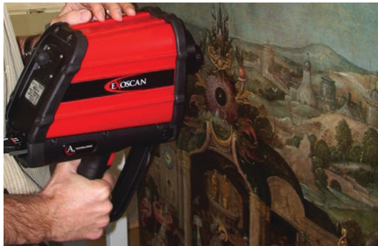
Agilent 4100 ExoScan FTIR analyzing a painting by H. Bosch. Photo courtesy of the Glasgow Museum.
