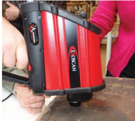
Figure 3. The handheld Agilent 4100 ExoScan FTIR is used to follow the cleaning process of a 17th century painting
