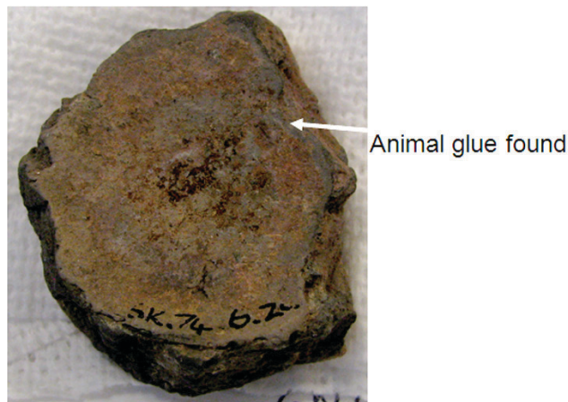
Figure 6. The exterior and interior surfaces of a pottery shard were examined using the Agilent 4100 ExoScan FTIR with Diffuse Reflection sampling accessory
