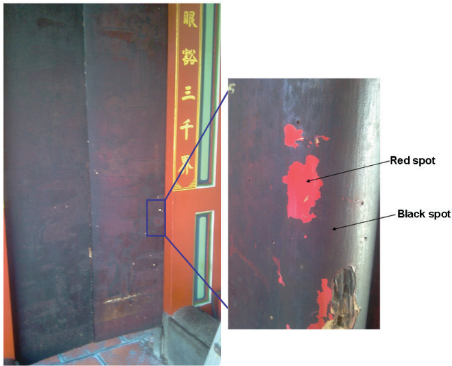
Figure 1. The doors of this temple were analyzed by the Agilent 4100 ExoScan FTIR handheld analyzer equipped with Diffuse Reflectance sampling accessory
