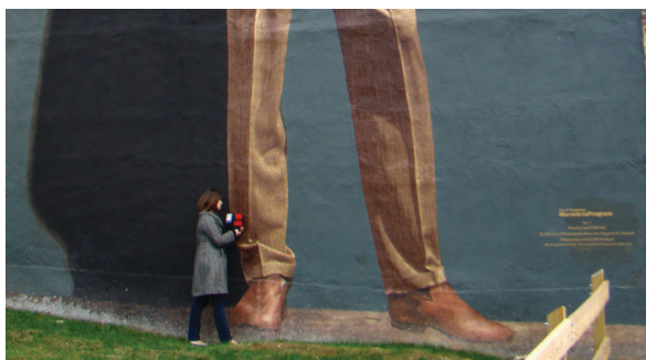
Figure 12. The Agilent 4100 ExoScan FTIR will be used to evaluate the condition of the “Dr. J.” mural to determine when re-coating/restoration is required.
