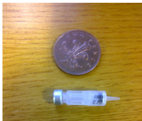
Figure 3 – ITSP coconut charcoal cartridge
